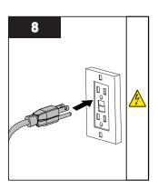
Restore power and connect the other devices such as solenoid, junction box and remote alarms.
