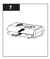
• Connect the sensor cable to the controller.
