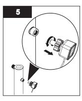
Remove the old sensor from UV chamber.
