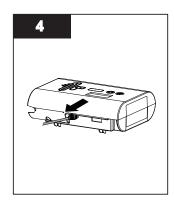
Disconnect the sensor cable from the controller.
